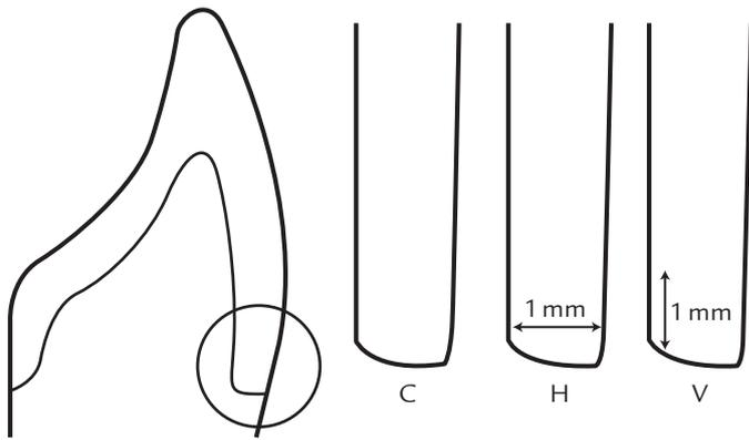
**1** Different designs of zirconia coping tested. Conventional zirconia-ceramic (C), zirconia-ceramic crowns with horizontal facial reduction of the zirconia coping (H), zirconia-ceramic crowns with additional vertical facial reduction of zirconia coping (V).
