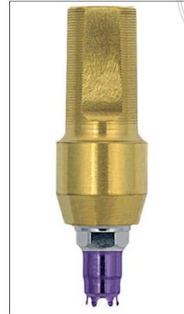
**Fig 2** Control abutment: GingiHue IAPP452G straight (Biomet 3i) with 2.0 mm collar height, profile 5.0 mm and platform 4.1 mm.
